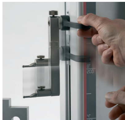
Fig. 1: Move the measuring slide manually in the direction of the measuring object.
